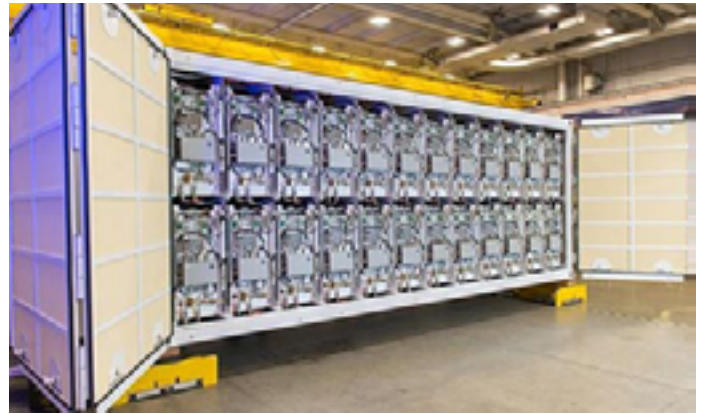
This device stores vast amounts of electricity and pumps it into the railgun in an eyeblink.
