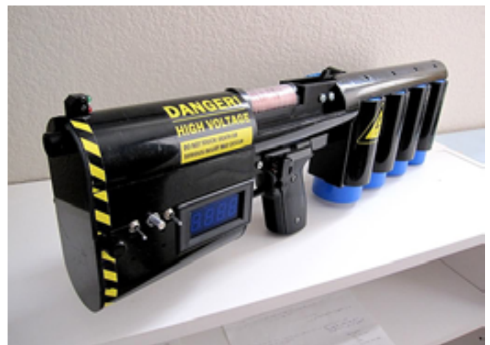
The coilgun uses many yards of copper wire, wound into tight coils, to fire a steel bullet.
