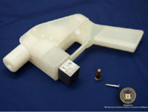
The infamous 'Liberator' 3D printed gun. Note the added block of metal to 'legalize' this gun.
