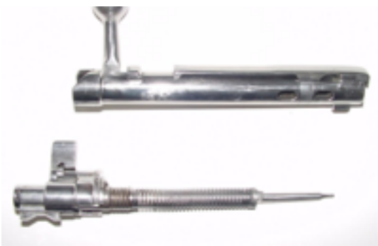
Needle gun bolt action and firing pin Licensed under Public Domain via Wikimedia Commons.
