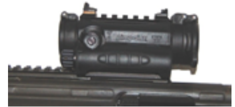
Reflex sights show a virtual red dot on target.
